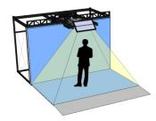
The **VisCube C1<sup>™</sup>** and **VisCube C2<sup>™</sup>** are **low cost** subsystems of the VisCube C4 CAVE immersive virtual reality system. The VisCube C1 features a large rear-projection wall. The VisCube C2 features a large rearprojection wall and a front projected floor. These systems are configured as turn-key immersive virtual reality systems, complete with a tracking system and graphics workstation. See options below.
