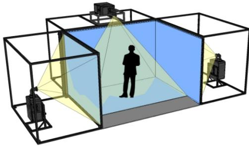
The **VisCube C4-4KU™** is a high resolution CAVE immersive virtual reality system. It features rear-projection walls and a front projected floor. The 12' wide front wall and floor allow more viewers in the space than a standard 10' wide CAVE configuration. The VisCube C4-4KU is configured as a turn-key immersive virtual reality system, complete with a tracking system and graphics workstation. See datasheet below.
