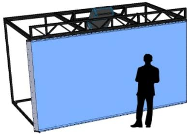
The **VisWall™ 4K** is a high resolution PowerWall display wall. The VisWall-4K features a large rear-projection wall. This system can be configured as a standalone display or as a turn-key immersive virtual reality system, complete with a tracking system and graphics workstation.
