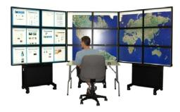
The **VisWall-LCD<sup>™</sup>** is an affordable and scalable high resolution display achieved by tiling LCD flat panel displays. High resolution panels with minimum bezels are used. However, for seamless display, the VisWall product (projector based) is more appropriate.
